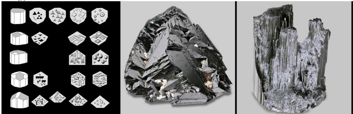
Figure 2. Left: overview of etching pits and hillocks on different tourmaline faces, middle: corroded schorl from Skardu (3.5 cm wide), right: deeply eroded schorl, from Skardu with portions of rim layer intact, 3 cm wide
