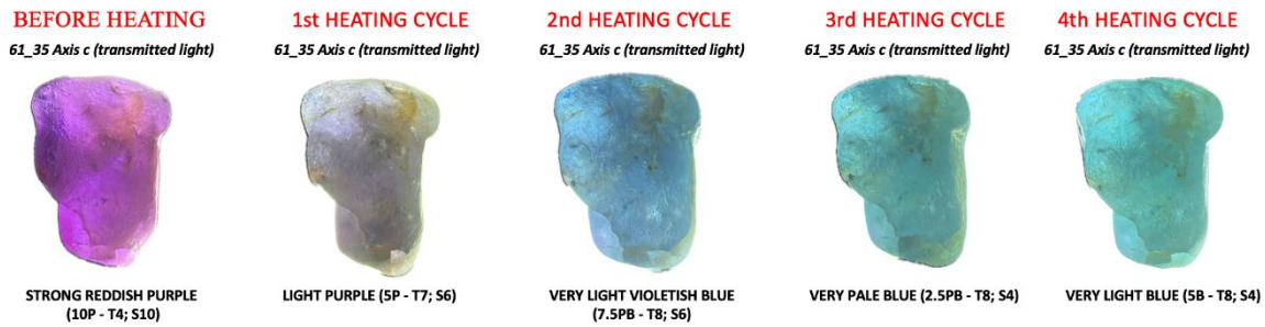
Figure 1: Heat treatment of a Cu-bearing violet tourmaline in a reducing environment, with increasing temperatures at each heating cycle, until the desired color is achieved.
